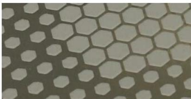
Figure 12: Application of PCM phase change material on SEMITRANS®10/SEMITRANS®10+ baseplate and inhomogeneous honeycomb structure.
