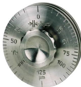
Figure 9: Recommended gauge to measure thermal paste thickness
