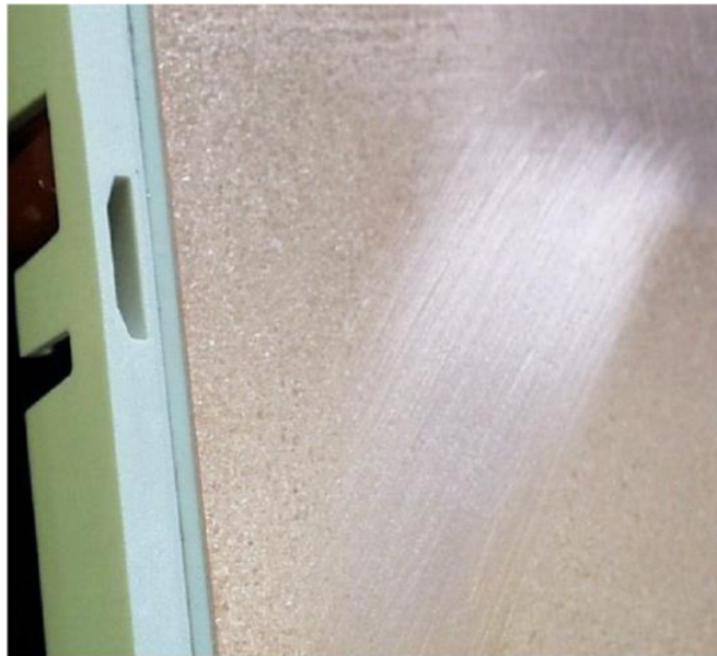
Figure 4: SKiM bottom surface after rework
