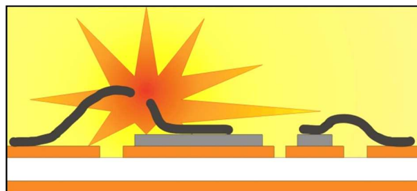
Figure 12: Sketch of high-energy plasma caused by melted off bond wire
