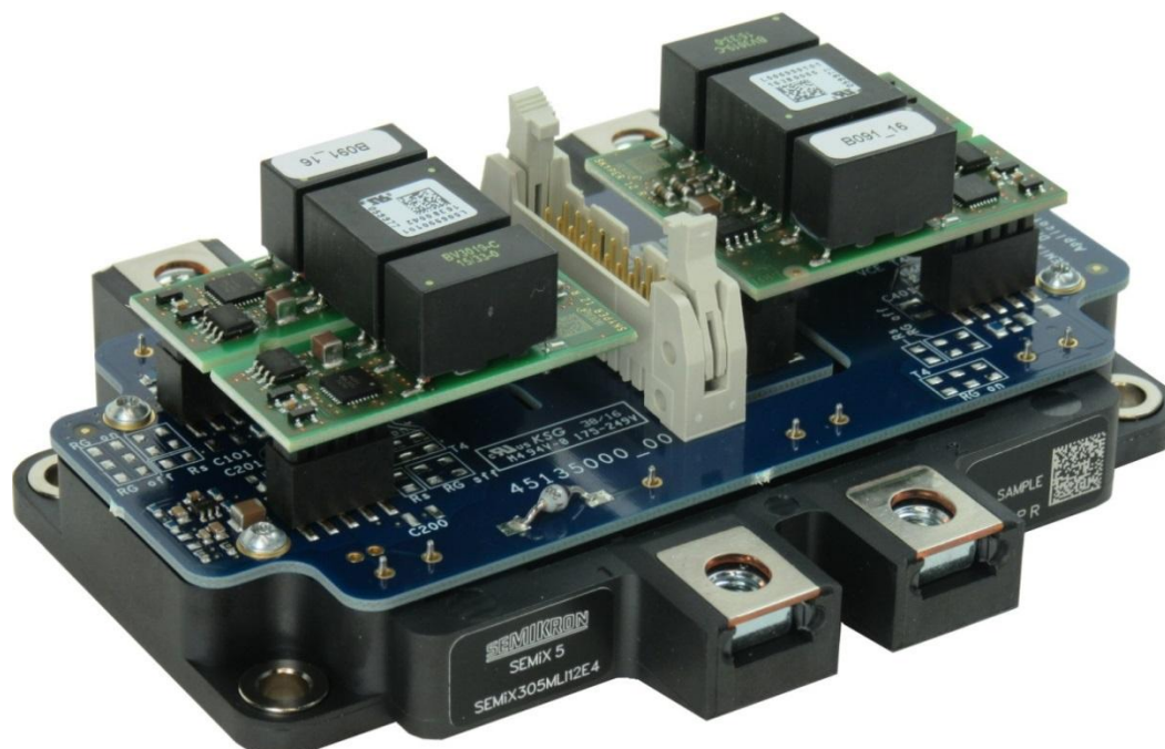
Figure 4: SEMiX5 1200V MLI SKYPER12 Driver Board bird's eye view
