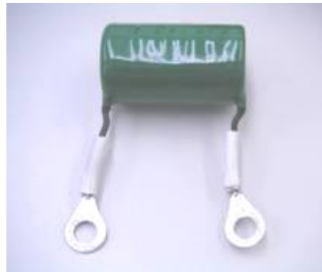
Fig. 8-12 Non-recommended snubber (too high a stray inductance).
