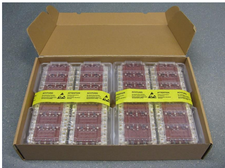
Fig. 11-2 Cardboard box with SKiM in transparent ESD tray, dimensions: 580 x 360 x 110 mm 3 (l x w x h)
